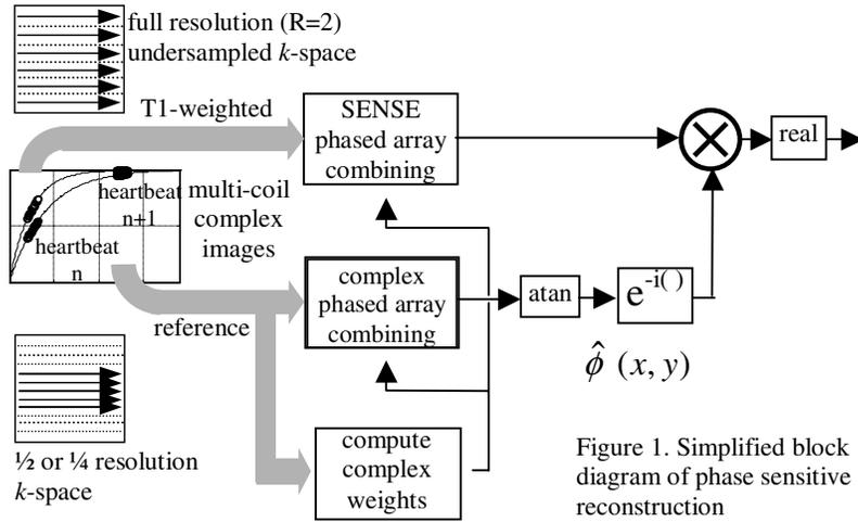
Figure 1. Simplified block diagram of phase sensitive IR reconstruction
