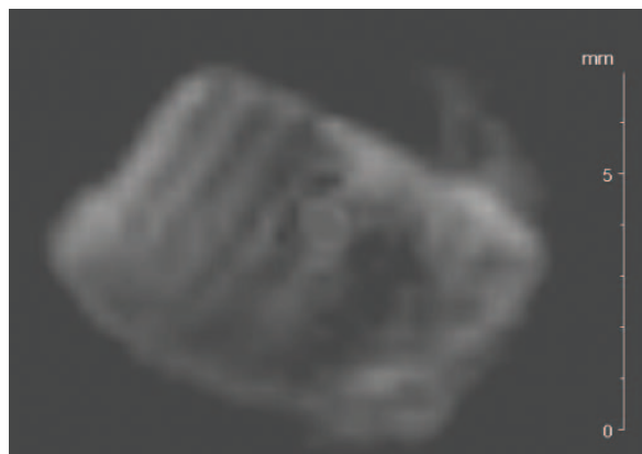
Figure 2. T2^* -weighted SPI image of an irradiated composite disk. Dark stripes indicate the solidification process under the brass grid (half period a=500\mu\text{m} ) to estimate the resolution obtainable.
