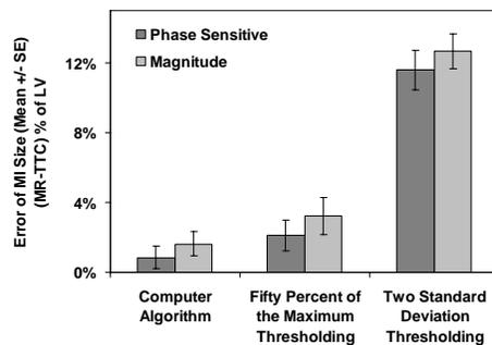
**Figure 5.** Average errors of infarct size measurement in units of percent of the LV mass for phase sensitive and magnitude MR images. The computer algorithm produces less than 2% average error for both phase sensitive and magnitude images. Fixed thresholding methods (fifty percent of the maximum and two standard deviation) consistently overestimated the infarct size compared to the computer algorithm.
